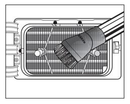
Remove any visible soiling carefully with a vacuum cleaner using a dusting brush or a narrow crevice nozzle.
